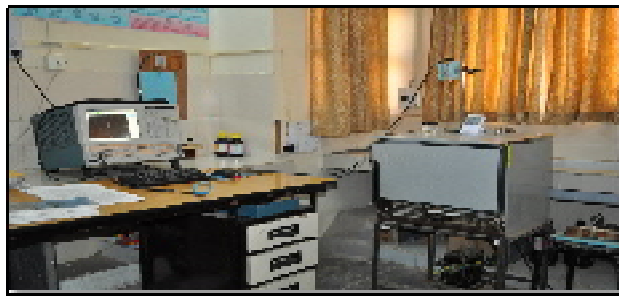
Fig. 9 TDR setup with temperature controlled system
