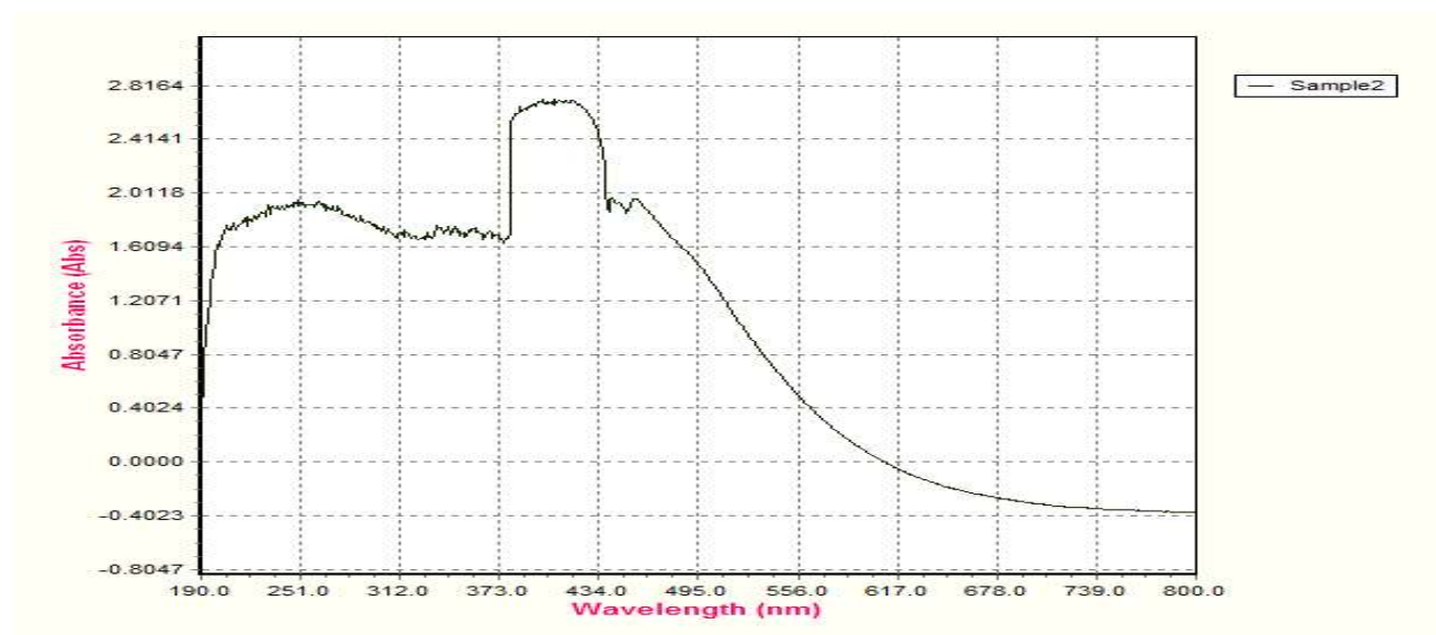
Figure-2: Electronic absorption spectrum of synthesized Mn (II) complex
